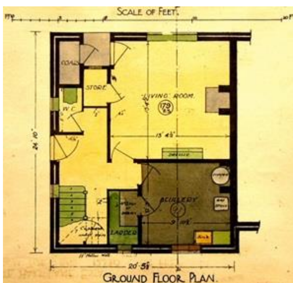
Fig. 10: White Hart Lane, Type "D" end of terrace, ground floor (LMA ref: LCC/AR/HS/03/056)
